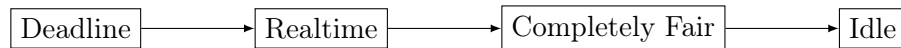
Figure 3: Order of scheduler submodules in the Linux kernel v4.13 with SMP disabled.
