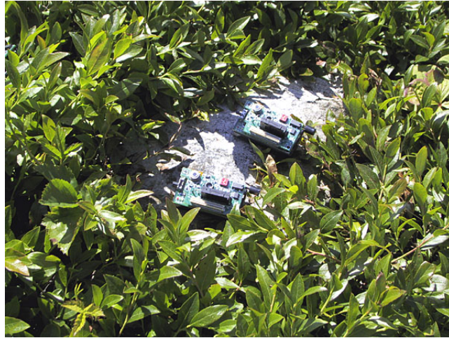
Figure 1.3: Two Berkeley sensor motes deployed on Great Duck Island. ( Image taken from [gre] )
