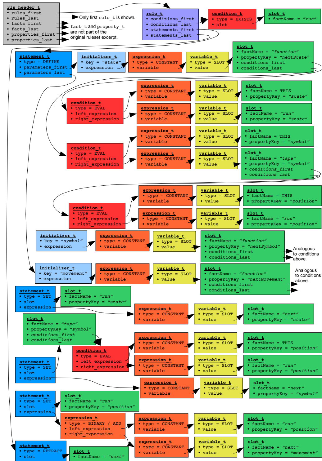
Figure 5.4: Bytecode data structure derived from the AST in Figure 5.3. Some redundant parts have been omitted for readability. Note how similar data is duplicated in several places within the data structure.
