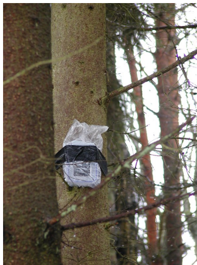
Figure 1.4: A ScatterWeb Embedded Sensor Board (ESB) node part of the Heathland Experiment. ( Image taken from [hea] )
