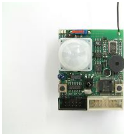
Figure 1.5: ScatterWeb Embedded Sensor Board (ESB). (Image taken from [sca])
