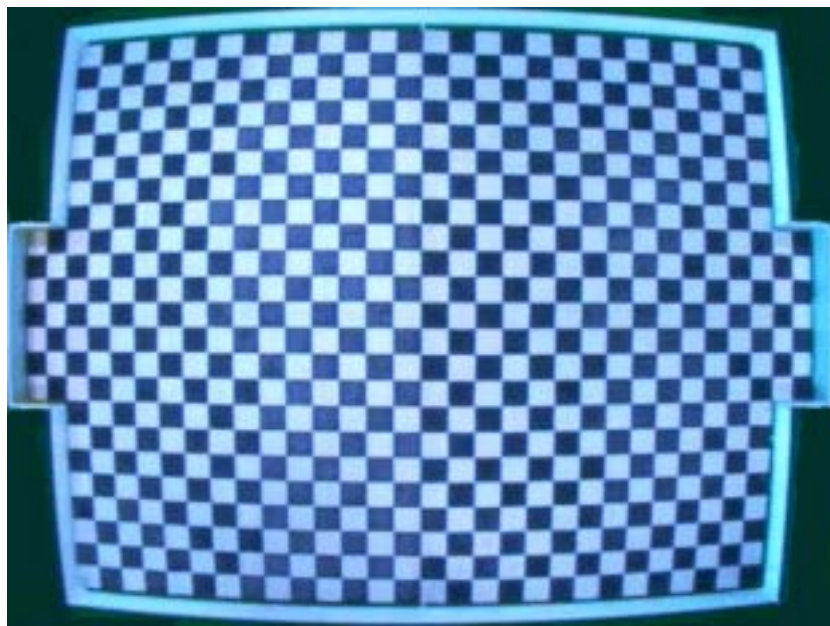
Figure 4: The checkerboard pattern used by the Cornell team to calibrate the camera
