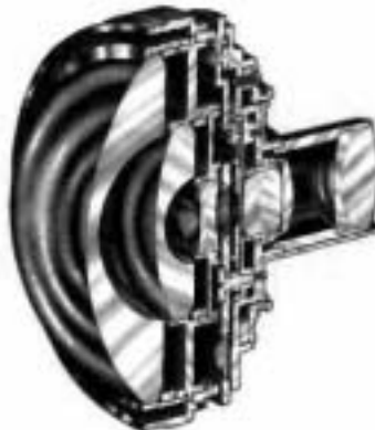
Figure 5: Stack of lenses used in the Nikkor fisheye
