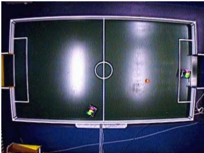
Figure 2: An example of barrel distortion from the wide angle
