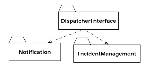
A complex system can be decomposed into subsystems, where each subsystem is modeled as a package
