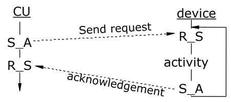
• The device can be regarded as a processor that executes exactly one thread. No switching. Active waiting for requests.
