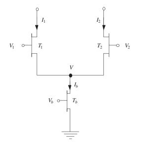
Fig. 18.7. Transconductance amplifier (Mead 1989)
