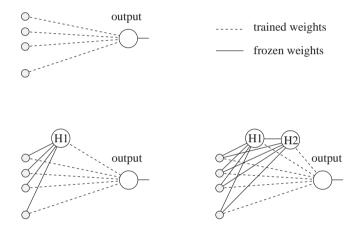
Fig. 16.1. The cascade correlation architecture
