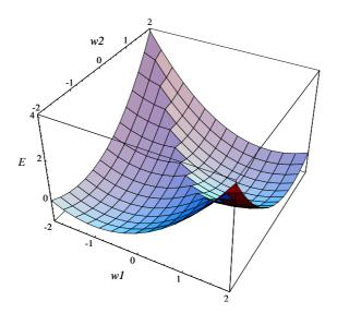
Fig. 5.8. Energy function of two two-dimensional clusters
