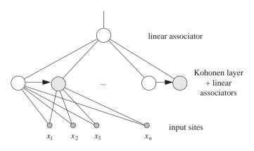
Fig. 16.7. Extended counterpropagation network
