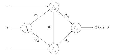
Fig. 1.15. Functional model of an artificial neural network
