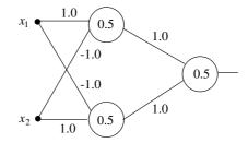
Fig. 6.2. A three-layered network for the computation of XOR
