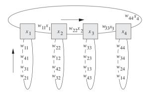
Fig. 18.15. Systolic array computing the product of W and x
