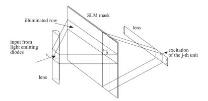
Fig. 13.21. Optical implementation of a Hopfield network
