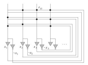
Fig. 13.20. Electrical implementation of a Hopfield network
