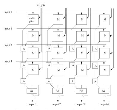
Fig. 18.14. Systolic array for 4 scalar product chains
