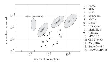
Fig. 18.1. Performance and capacity of different implementations of neural networks and performance requirements for some applications [Ramacher 1991]
