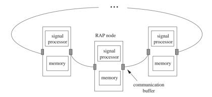
Fig. 18.17. Architecture of the Ring Array Processor
