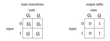
Fig. 2.22. State tables for a binary delay
