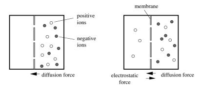
Fig. 1.4. Diffusion of ions through a membrane
