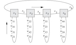
Fig. 18.16. Systolic array computing the product of the transpose W and x
