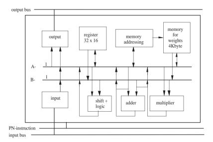
Fig. 18.21. Structure of a processor node
