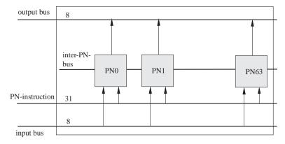
Fig. 18.20. CNAPS-Chip with 64 processor nodes (PN)
