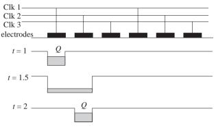
Fig. 18.9. CCD transport band
