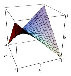
Fig. 13.5. Energy function of a flip-flop
