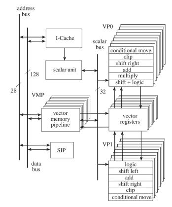
Fig. 18.19. Torrent block diagram [Asanovic et al. 95]
