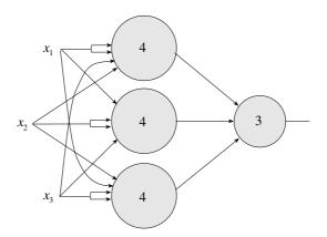
Fig. 2.27. A fault-tolerant AND built of noisy components
