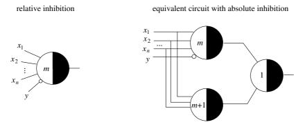
Fig. 2.19. Two equivalent networks
