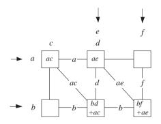
Fig. 18.12. Planar systolic array for vector-matrix multiplication
