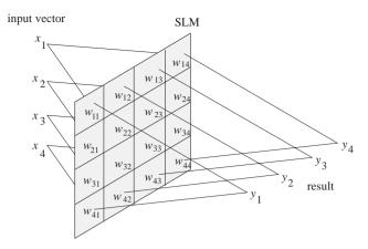
Fig. 18.23. Matrix-vector multiplication with an SLM mask
