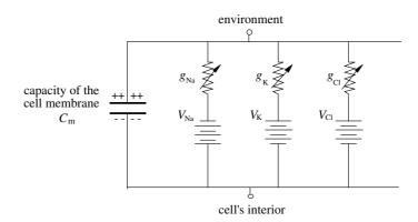
Fig. 1.6. The Hodgkin–Huxley model of a cell membrane
