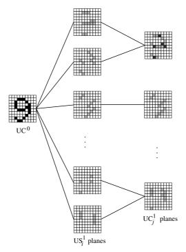
Fig. 3.16. The architecture of the neocognitron
