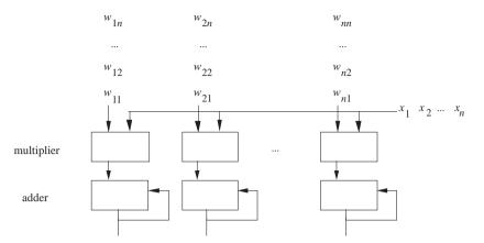
Fig. 18.18. SIMD model for vector-matrix multiplication
