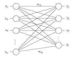
Fig. 13.1. Example of a resonance network (BAM)
