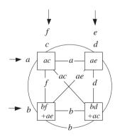
Fig. 18.13. Systolic array with toroidal topology
