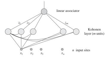
Fig. 16.10. Hybrid network with RBFs
