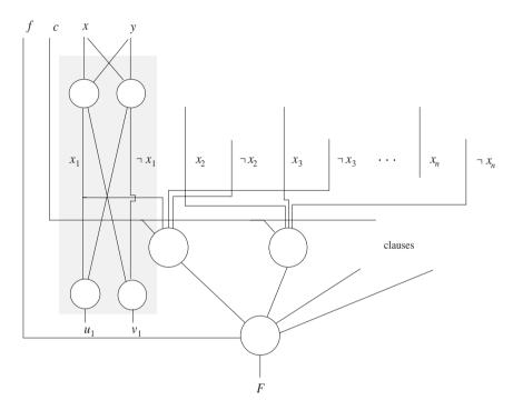
Fig. 10.11. Equivalent network for the 3SAT problem with AND-OR units
