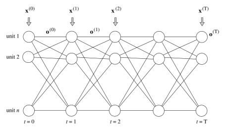
Fig. 7.24. Backpropagation through time
