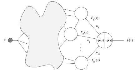
Fig. 7.15. Backpropagation at the last node
