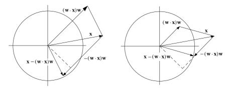
Fig. 5.18. The two cases in Oja's algorithm
