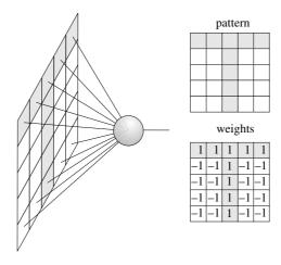
Fig. 3.13. Feature detector for the pattern T
