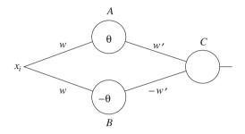
Fig. 10.13. Network to compute even functions
