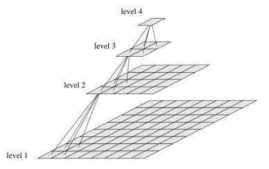
Fig. 3.14. Pyramidal architecture for image processing
