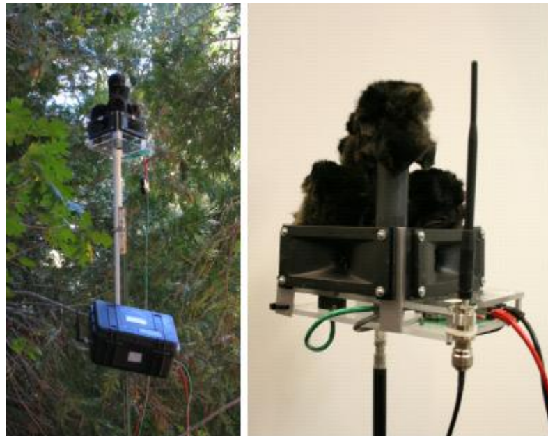
Abbildung 4: Acoustic Embedded Networked Sensing Box [4]
